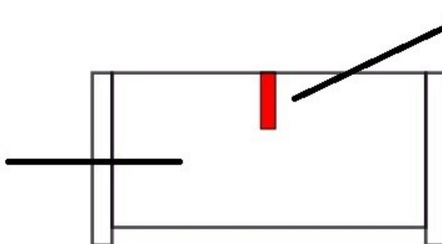
Vertical line 10cm by 2.5cm on the centre back of the wheelchair seat back, on the outer side. The line is to be marked in a contrasting colour to the seat back.
